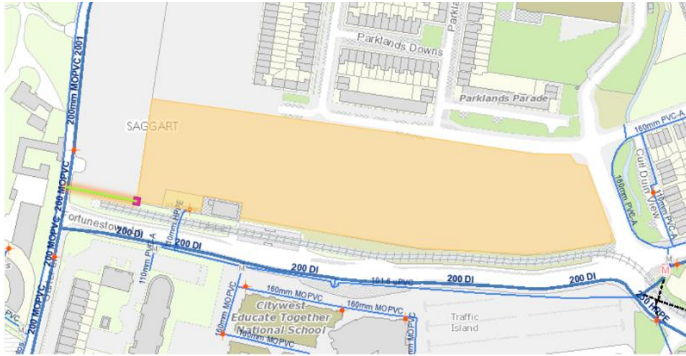
Figure 1: Site boundary, 200mm connection main and meter
