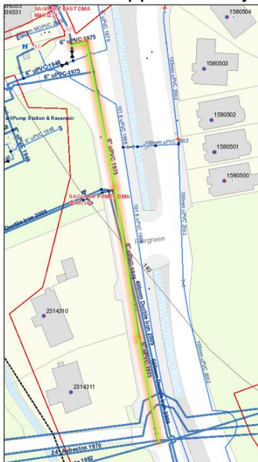
Figure 2: Existing 6" uPVC main to be upsized to 300mm DI (coordinates: 303830, 226337)).
