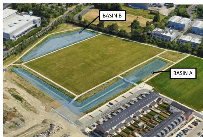
Figure 3-1: Existing Open SuDS Basins which receive site run-off,
